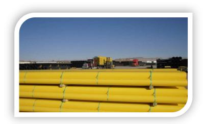
DRISCOPLEX® MDPE Pipe is manufactured to meet your needs in compliance with ASTM D2513, NSF Gas and DOT 49 CFR 192. Selected sizes conform to CSA B137.4 and UPC product standards.
