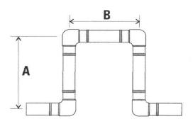
Figure 5: Conventional Expansion Loop
