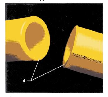
4. Proper melt ends after heat soak
