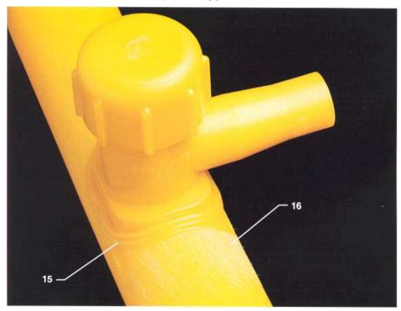
15. Proper melt, pressure and alignment.
