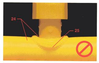
24. Melt bead is above base of fitting; Main not prepared25. Excessive melt bead size
