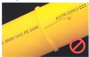
12. No melt bead caused by incomplete face off
