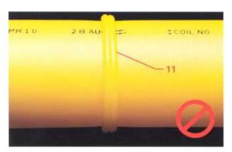
11. Excessive melt and/or excessive pressure
