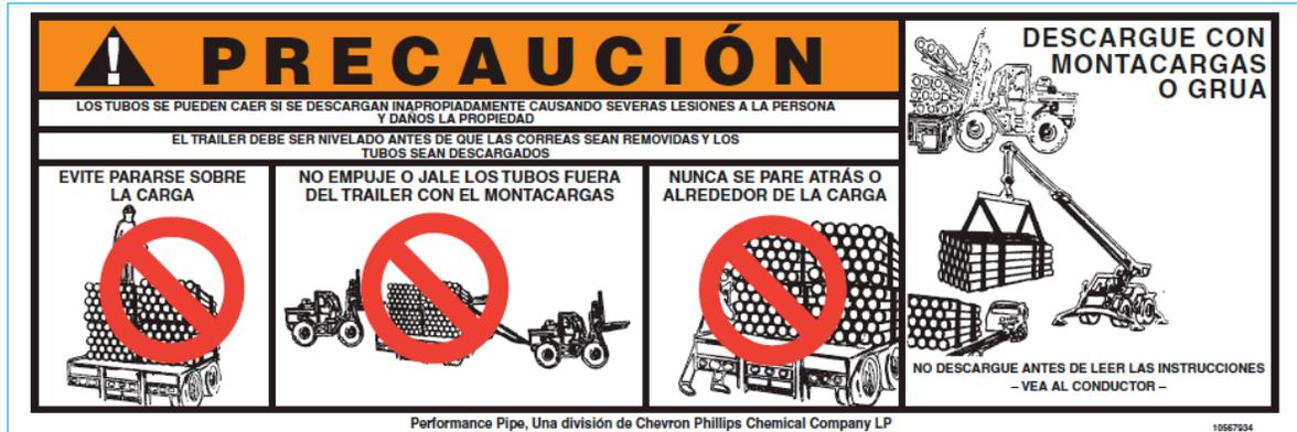
FOR BULK PACKS, SOFT PACKS AND HARD SIDED BUNDLES. TO BE ATTACHED ON THE LOWER PACKS ON EACH SIDE OF THE TRUCK
