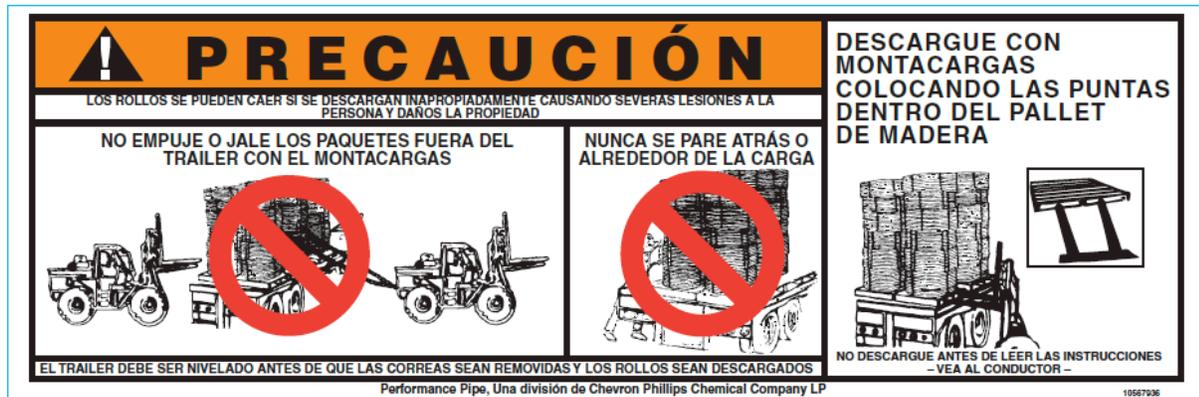
FOR COILED PIPE IN SILO PACKS. ATTACH THE LABEL TO A MINIMUM OF TWO SILO PACKS ON EACH SIDE OF THE LOAD.
