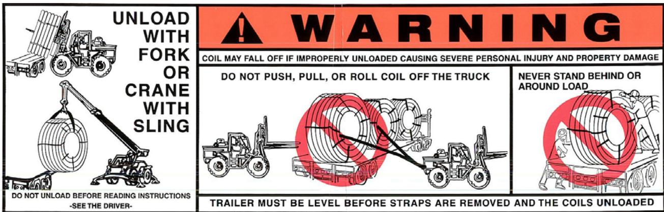
FOR VERTICAL COILS, TWO LABELS ARE TO BE ATTACHED TO ONE COIL ON BOTH SIDES OF THE TRUCK.
