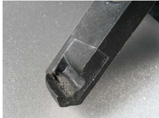
Figure 5. Unusual ductile failure of tab on thermostat housing.
