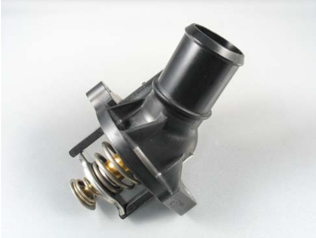
Figure 1. Thermostat housing showing the thermostat in place, held by the small tabs at the end of each arm.
